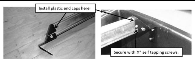
6. After the brackets and end caps are installed, the seat rail may be bolted into place with the 1/4" bolts, washers and nylock nuts using the previously drilled holes. Install plastic base and seat onto the rail. Use WD-40 or silicone to lubricate plastic seat base opening so it will go onto the aluminum rail easier.
