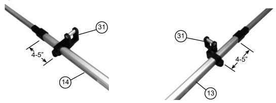
15. Slide middle main frame (Item 15) onto items 13 and 14 assembled in step 13 and lock together. Lubricate frame bars for best operation as shown in step 11.
